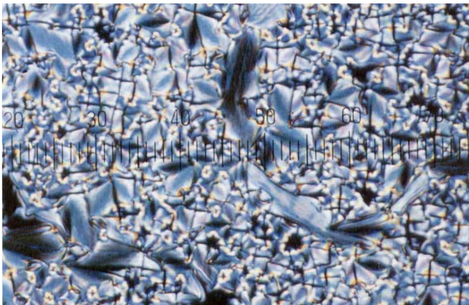
Figure 14. Fan-like textures of smectic A phase for PBU observed between crossed polars in the microscope ( \times 420 ) at 132^{\circ}\text{C} .
